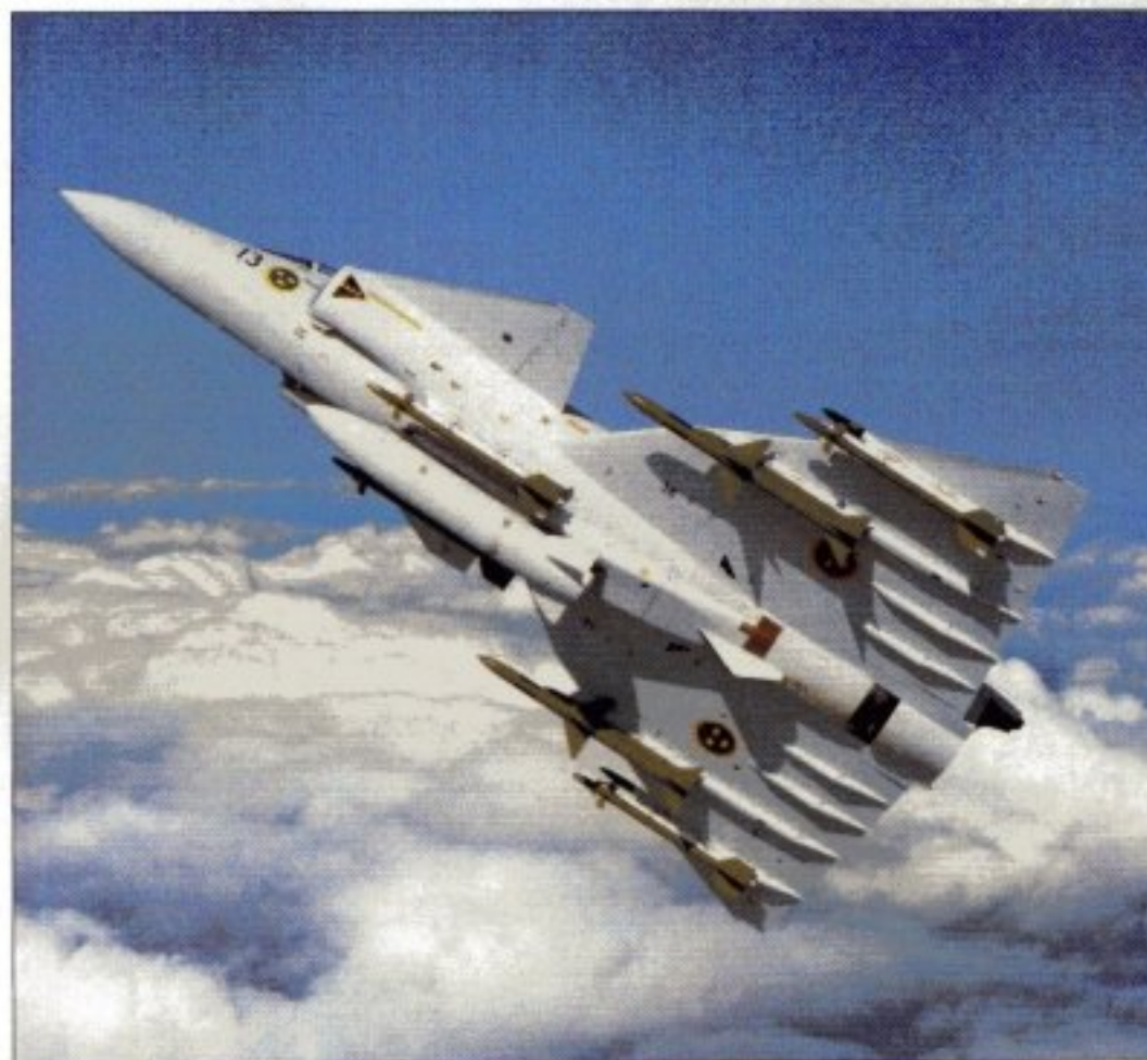
Above: The Viggen's large canard wing enables it to take off and land on very short runways. Below: A line-up of JA 37 Viggens from F17 at Kallings in southern Sweden, some of them with the unique camouflage pattern chosen for most Swedish military aircraft. Lennart Berns
