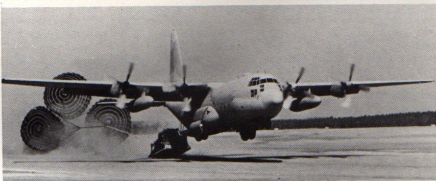
Hercules using the low altitude parachute system (LAPES) to make an emergency delivery of supplies
