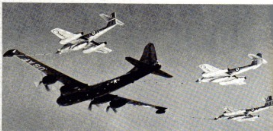
The USAF tested the probe and drogue system fitted to a B-29, here refuelling RAF Meteor F8s. FRL
