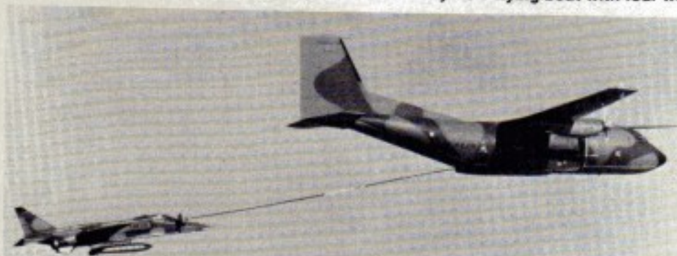
A French Air Force Transall refuelling a Jaguar using a Sargent-Fletcher centreline hose reel
