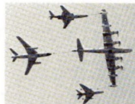
The USAF's Tactical Air Command had 3-point drogue units on the B-29s/KB-50s for AAR. Here an F-101 Voodoo, B-66 Destroyer and F-100 Super Sabre are all hooked up. PRM
