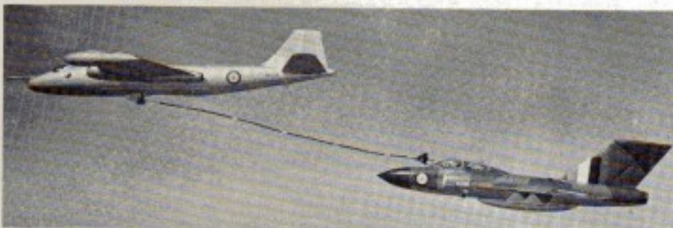
Trials were conducted by FRL's Canberra refuelling most of the RAF's front-line fighters, such as the Javelin. Russell Adams
