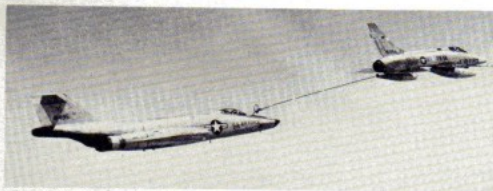
F-100 Super Sabre with a 'Buddy' refuelling system under the port wing supplying an RF-101 Voodoo
