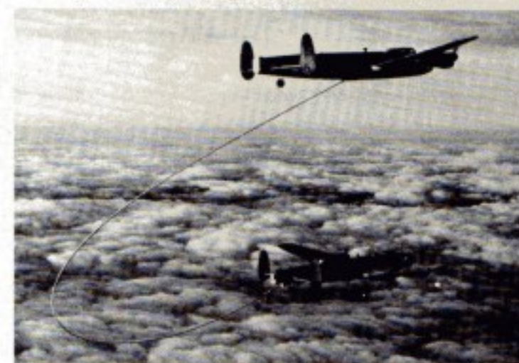
Avro Lancaster refuelling using the looped hose method during trials by Flight Refuelling Ltd.
