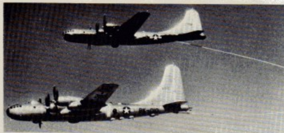
The USAF first used the looped hose method of AAR with its B-29/B-50 bombers of Strategic Air Command. USAF
