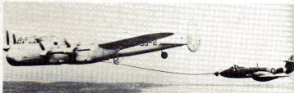
Flight Refuelling Ltd. invented the probe and drogue system for AAR of jet fighters. The first contact was made in April 1949 by this Meteor and Lancaster tanker. FRL
